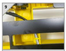
Secure the extension cables to the step using the 12 small cable ties. (PRO-PARK-AM10Y Shown)
