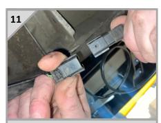
Connect the parking sensor cables to the original vehicle parking sensor connectors and use the larger cable ties to secure in place.
