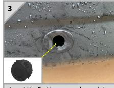
Insert the Parking sensor bungs into the OEM carriers to blank off the holes in place of the OEM Sensors. The bungs push in from the outside.
