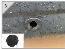
Insert the Parking sensor bungs into the OEM carriers to blank off the holes in place of the OEM Sensors. The bungs push in from the outside.
