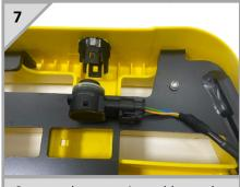
Connect the extension cables to the OEM sensors.
