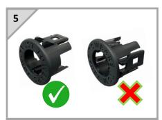
Ensure the carriers are the correct orientation before fitting them to the step.
