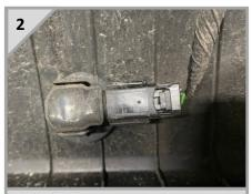
Remove the 4 OEM parking sensors from the rear bumper, leaving the carriers in the bumper.
